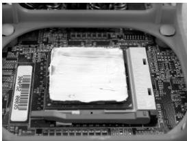
Figure 1. Apply the thermal tape(or grease) to provide better heat conduction between your CPU and cooling fan.
